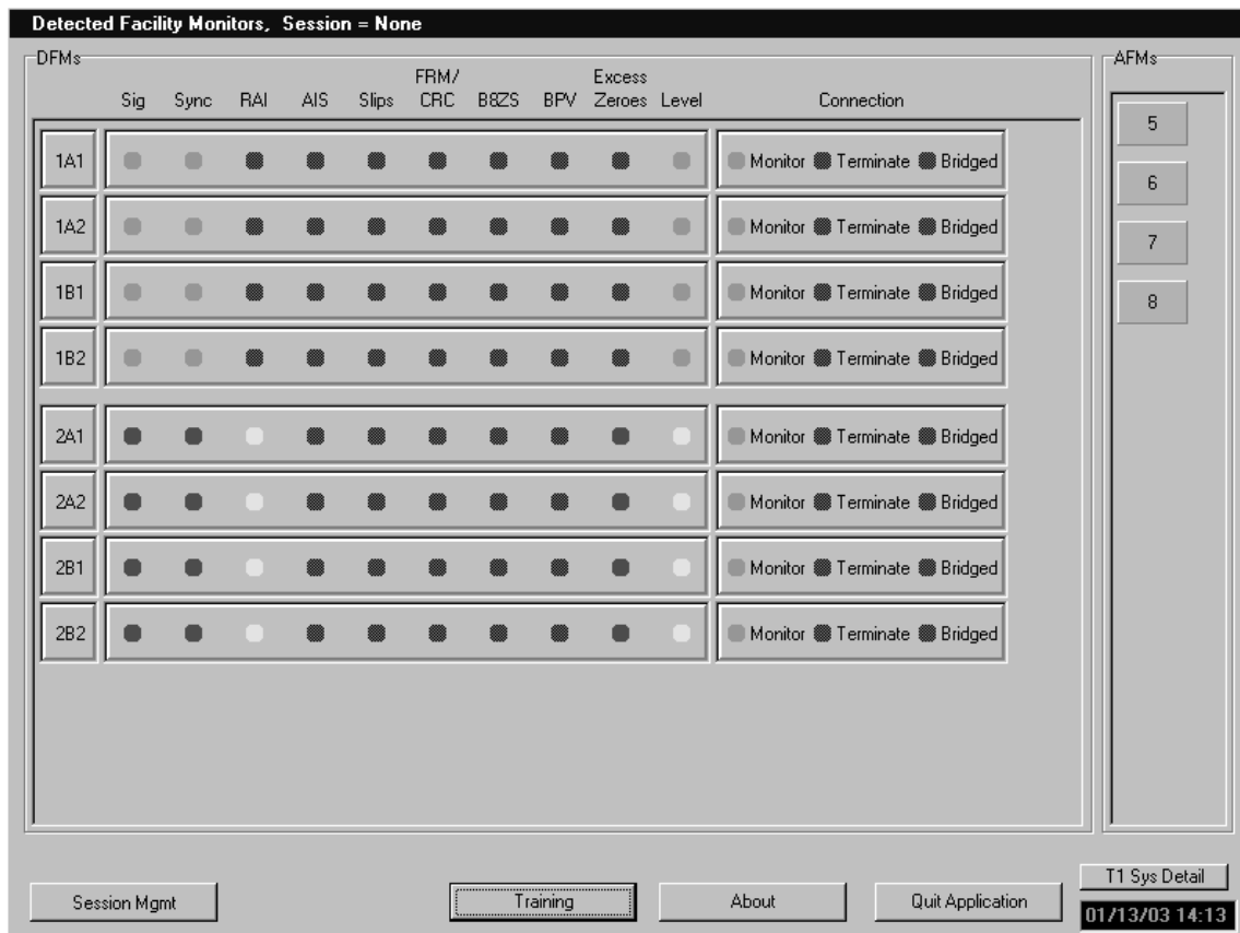
Figure 17. Detected Facility Monitors Window, CAS Mode; Shows One E2D With One E4AC5
