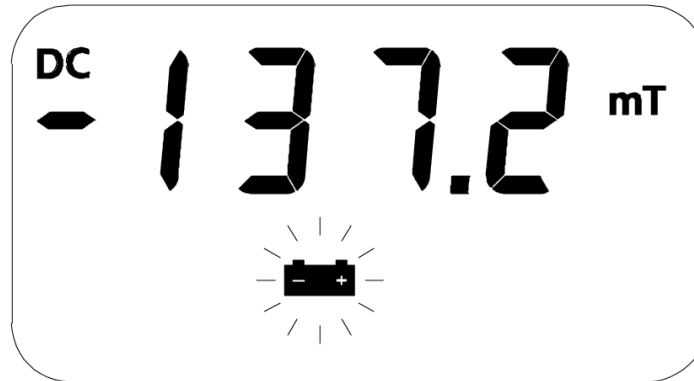
Figure 3-8 Low Battery Indication
