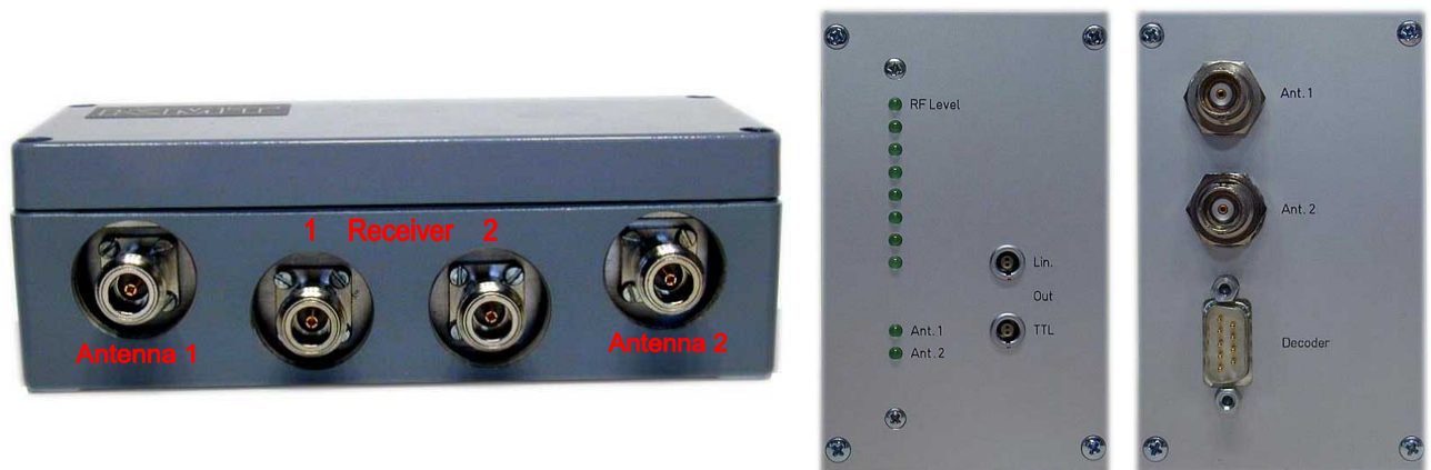
Connectors and indicators of the GHz converter and the diversity receiver
