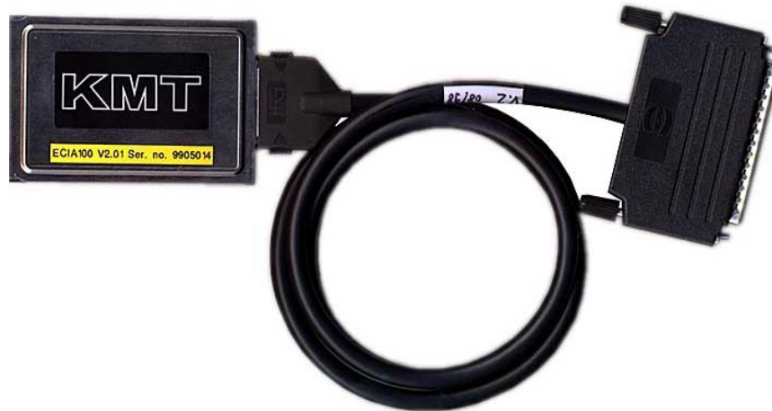
Digital interface ECIA100 for PCMCIA slots in notebook computers with cable (pin assignment equal to IF16)
