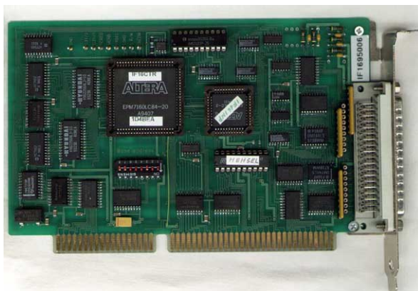
Digital interface IF16 for ISA slots in desktop computers, cable for analog decoders and pin assignment
