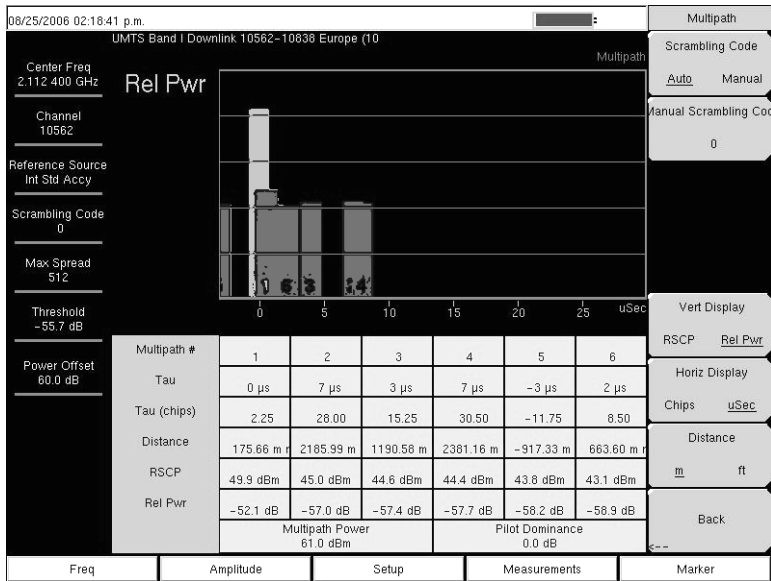
Figure 9-24. Multi-Path Power Measurement Screen Example
