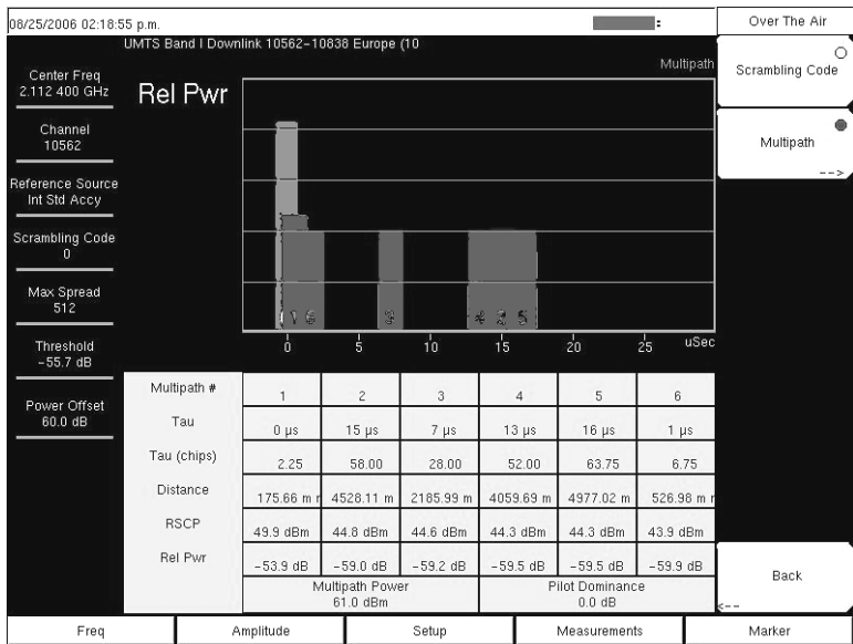
Figure 9-23. Multi-Path Power Measurement Screen Example
