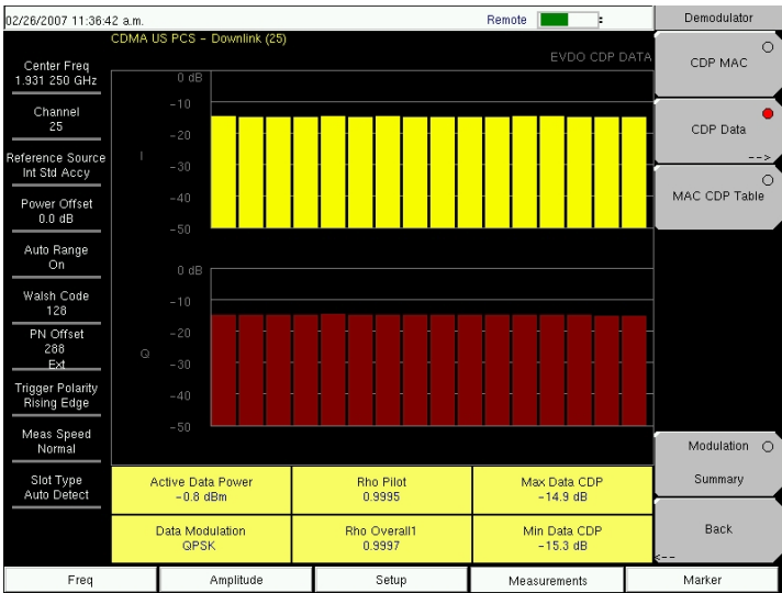
Figure 16-6. EVDO CDP Data Measurement Display
