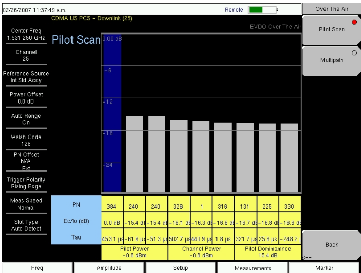
Figure 16-9. EVDO OTA Pilot Scan Measurement Display
