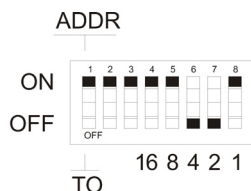
Figure 8 IEEE Interface Default DIP Switch Settings
