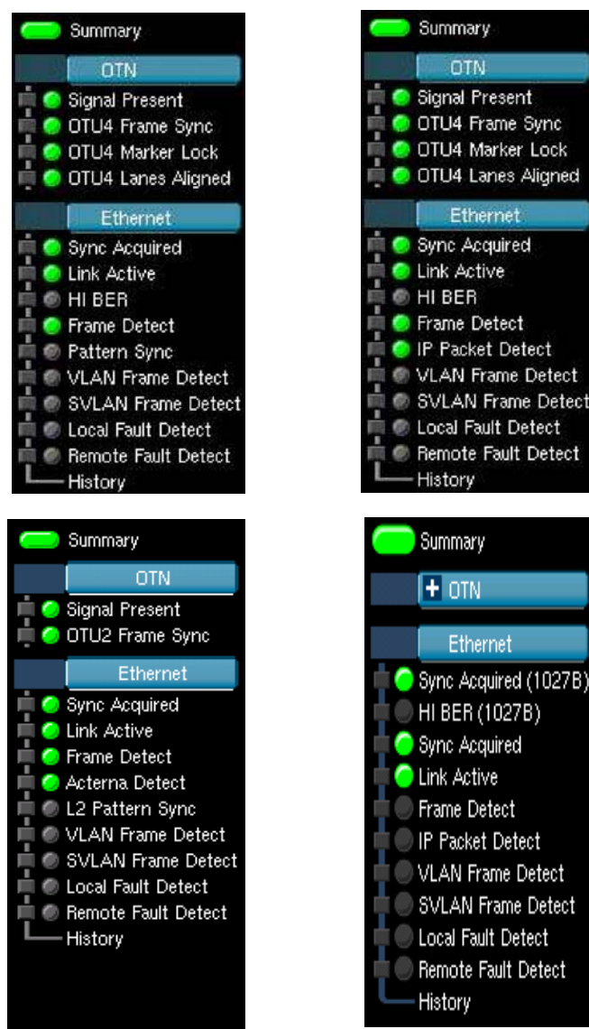
Figure 25 OTN LEDs (Ethernet payloads)
