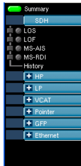
Figure 14 NextGen SDH LED categories (GFP Ethernet payload)
