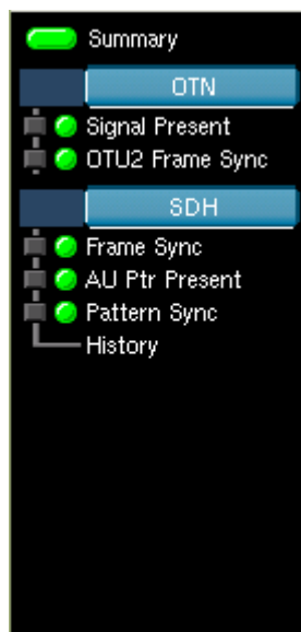
Figure 24 OTN LEDs (SDH payload)
