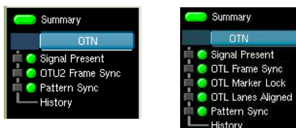
Figure 23 OTN LEDs (bulk BERT payloads)
