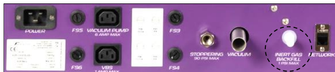
INERT GAS BACKFILL
