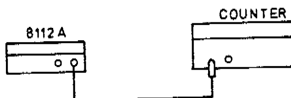
Figure 4-1. Equipment setup for PER performance test.
