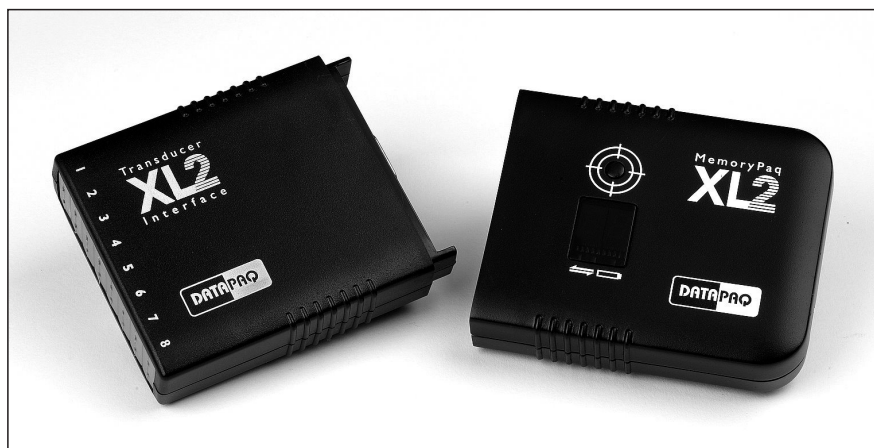
The basic XL2 logger: an eight-channel Transducer Interface (left, showing thermocouple sockets) and MemoryPaq (right).
