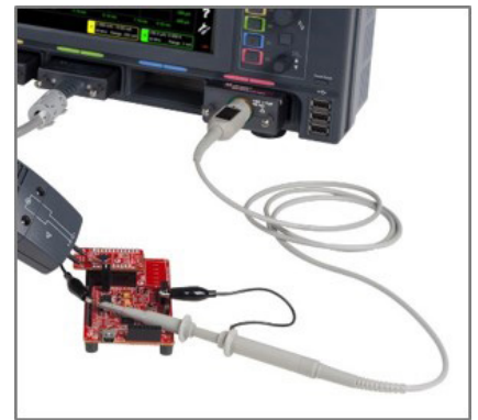
Figure 32. Example of voltage measurement using a passive probe
