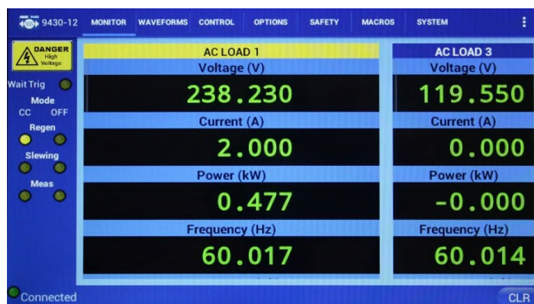
Monitor Screen showing a 9430 in split phase (2- \phi ) + 1 AC (1- \phi ) Configuration
