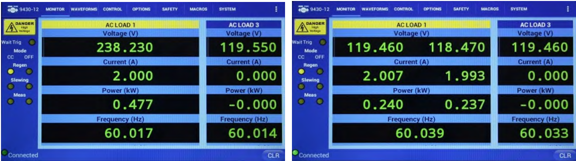
9430 Line-Line view for AC Load 1 Shown
