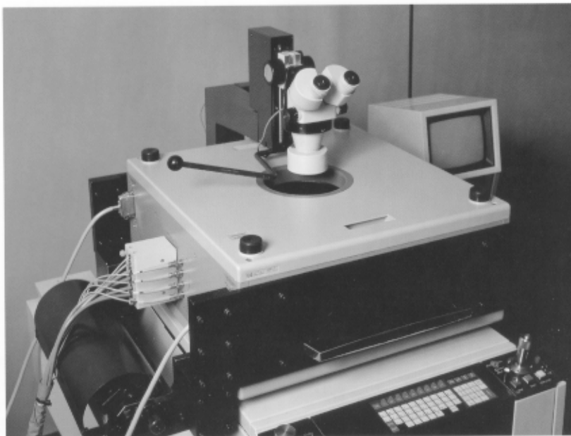
The HP 4089A 96-pin switching matrix mounted on a wafer prober.
